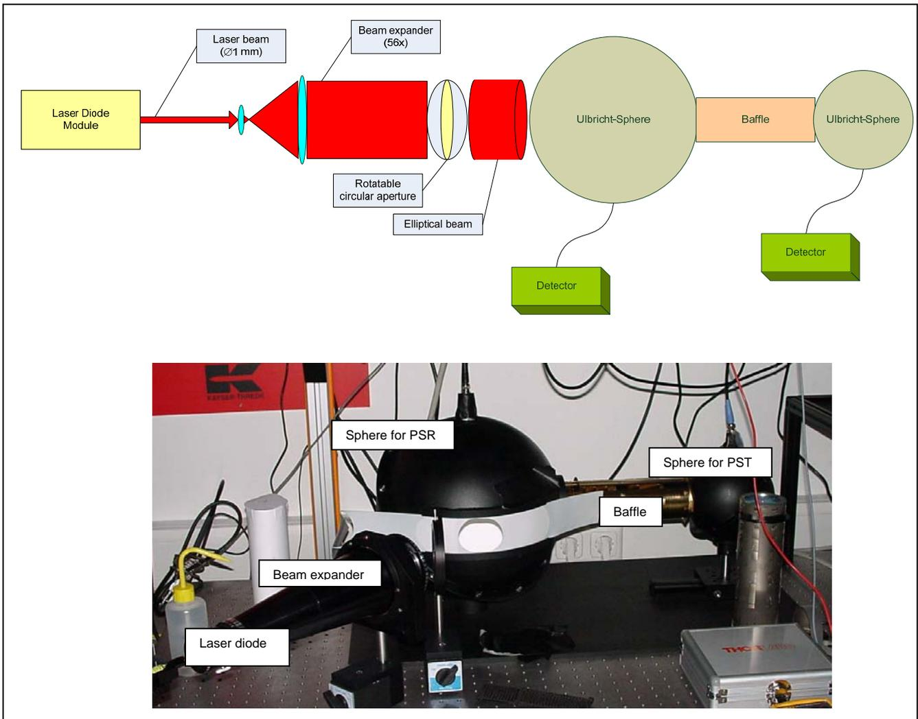
Figure 6: Test setup to measure the Point Source Transmittance (PST) and point source Reflectance (PSR).
