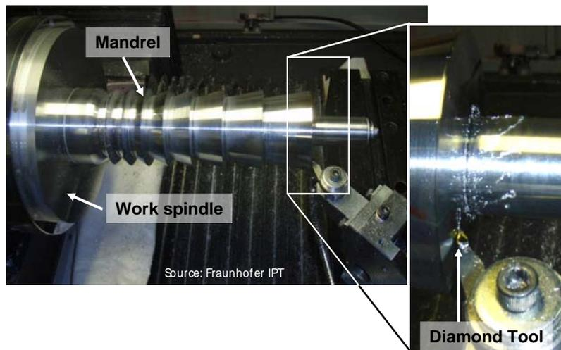
Figure 2: Diamond turning of mandrel. By courtesy of Fraunhofer IPT/Aachen.
