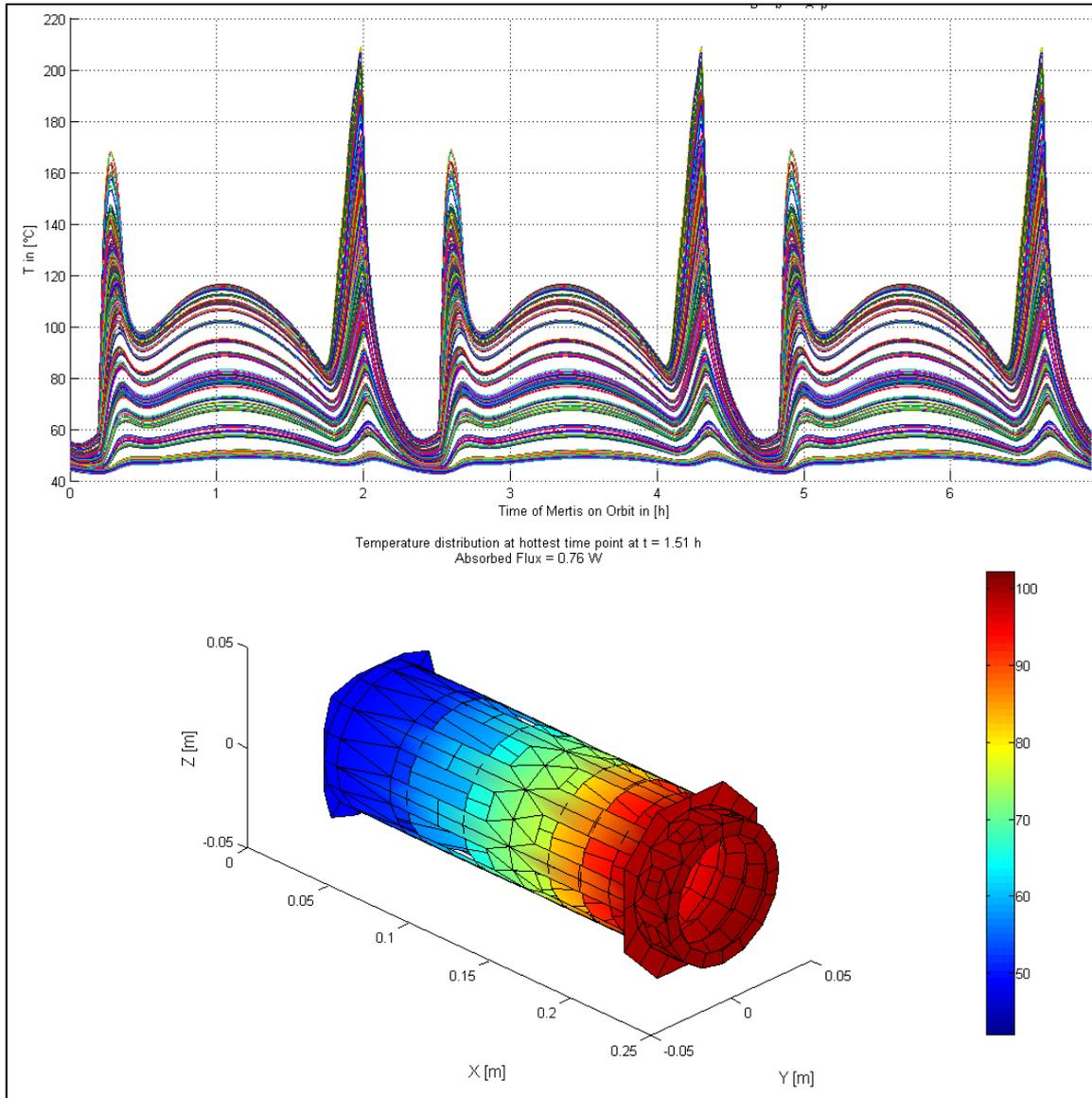
Figure 5: Simulated, thermal loads on a gold coated baffle during three orbits (upper curve). The upper, multiple curves show multiple thermal nodes on the baffle. The lower figure shows a snap-shot temperature distribution to show the gradient from the tip to the end of baffle.
