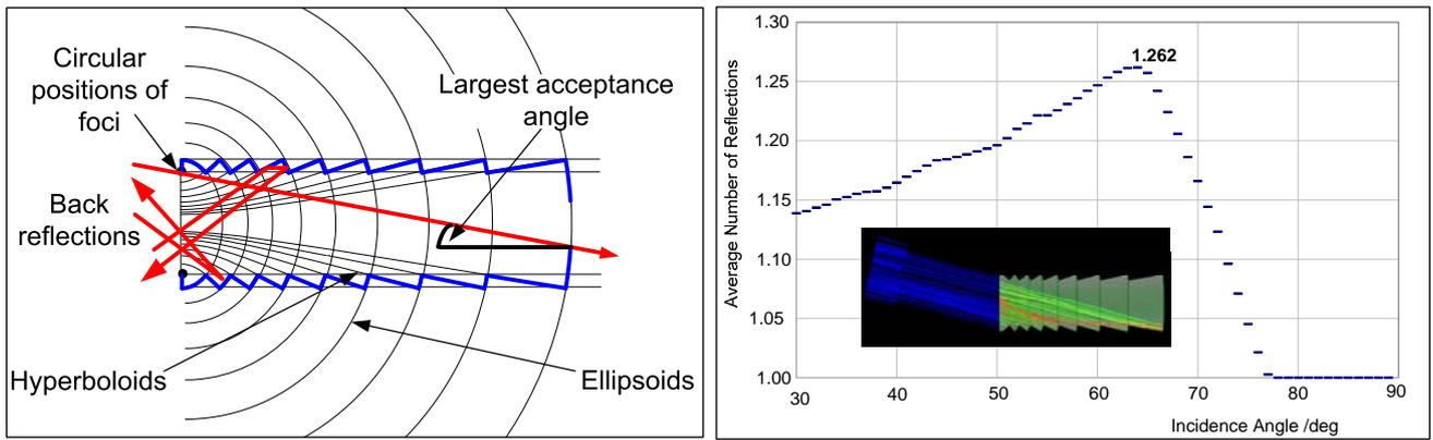
Figure 1: Consecutive ellipsoids and hyperboloids are leading to a minimum number of reflections.
