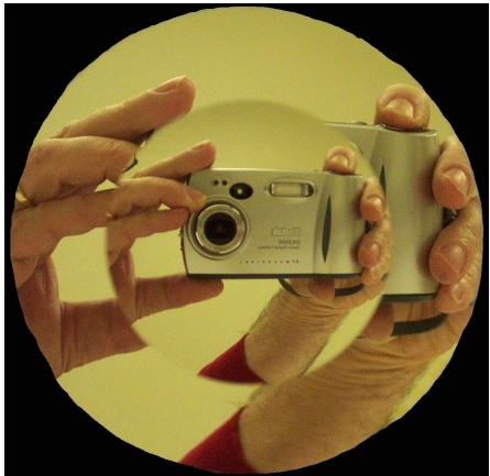
Figure 3: Gold faced electroformed NiColoy™ mirror
