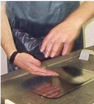
Electroformed foil being separated from the mandrel
